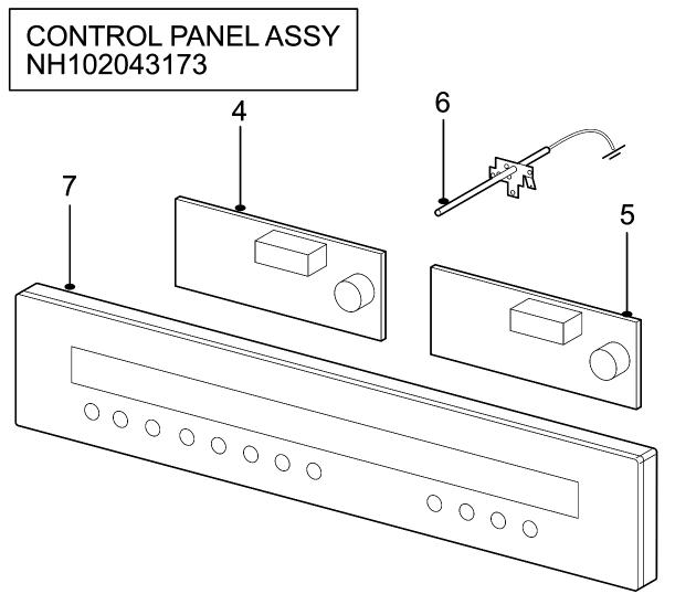
Control panel assy is a one peice assembly and includes: panel,on/off switch & knobs.
