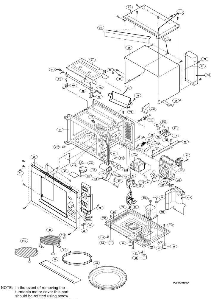
should be refitted using screw connection: 5028 14 53-00/6 (710)
