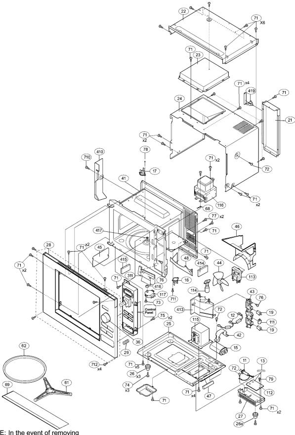
NOTE: In the event of removing the turntable motor cover this part should be refitted using screw connection: 5028 05 76-00/5 (71)
